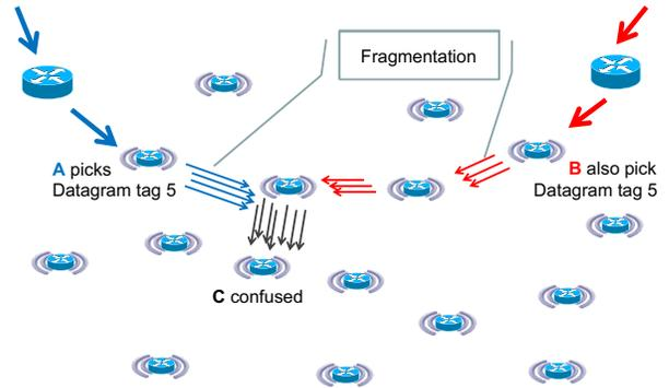
Fig. 7. Multiple simultaneous flows from different sources.
