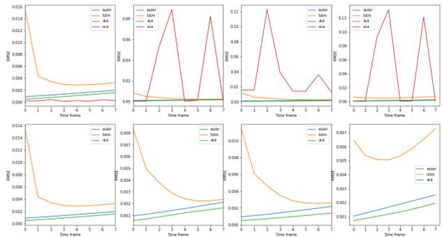
**Fig. 3.** RMSE for all the tested methods plotted against the considered prediction time step (top: with VCA baseline, bottom, without VCA baseline). From left to right: vegetation, metallic roofs, concrete, asphalt.
