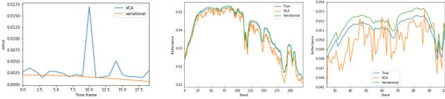
**Fig. 1.** RMSE of the endmember trajectory with known dynamical model compared to VCA frame-by-frame extraction (left). Endmember reconstruction with known dynamical model for the last frame ( $T = 20$ ), using VCA on each frame and variational data assimilation (middle). Zoomed version (right).
