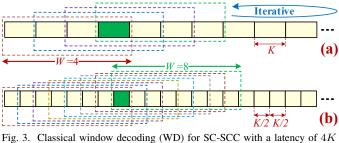
Fig. 3. Classical window decoding (WD) for SC-SCC with a latency of 4K bits. (a)  $\{W = 4, K, \mathcal{L} = 4K\}$  and (b)  $\{W' = 8, K' = K/2, \mathcal{L} = 4K\}$ .
