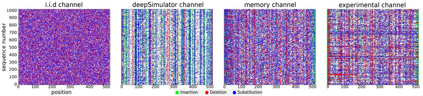
Fig. 1. Errors and types of errors observed on barcode03, for 1000 output sequences.
